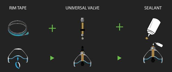
Install blue rim tape evenly across the inside of the rim while covering the spoke holes up to the sides.
